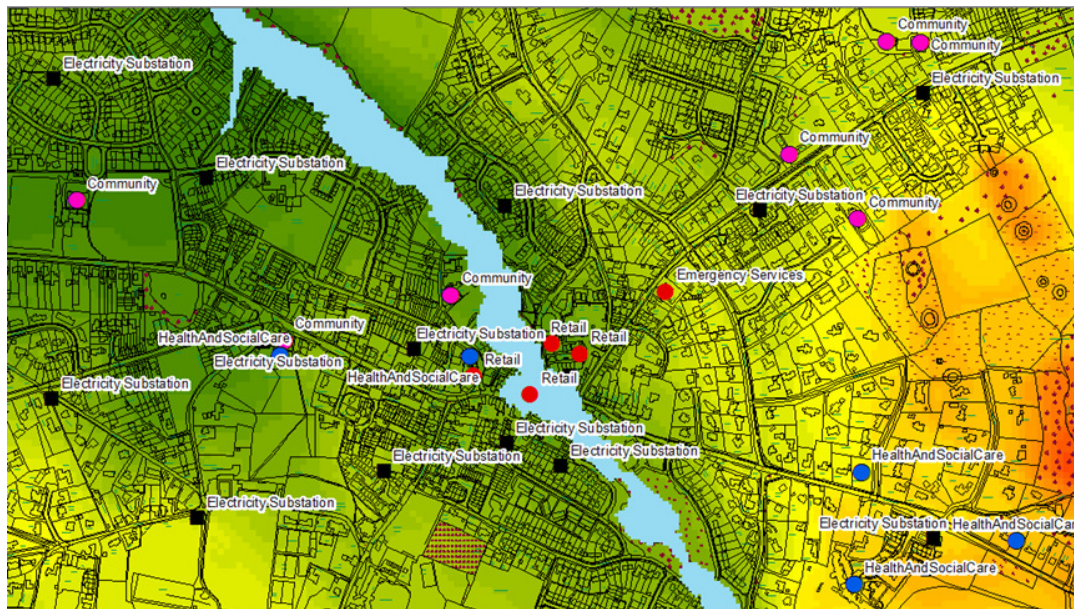
Figure 3.3 An example of a flood zone, electricity substations and demand nodes in 'Village Hub'.
