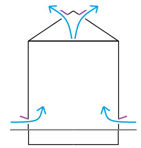
Thermal mass: Active rock storage Warm air is ducted from the top of the greenhouse into the rock bed beneath the greenhouse to be stored. At night, when the greenhouse cools, heat is supplied from the rock mass passively.
