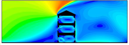
Low wind speed 0.4m/s •2 air changes per hour High wind speed 5m/s •30 air changes per hour
