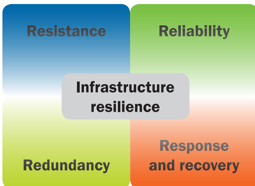
Figure 1 Cabinet Office framework of components of infrastructure resilience (from Cabinet Office and IUK, 2010)
